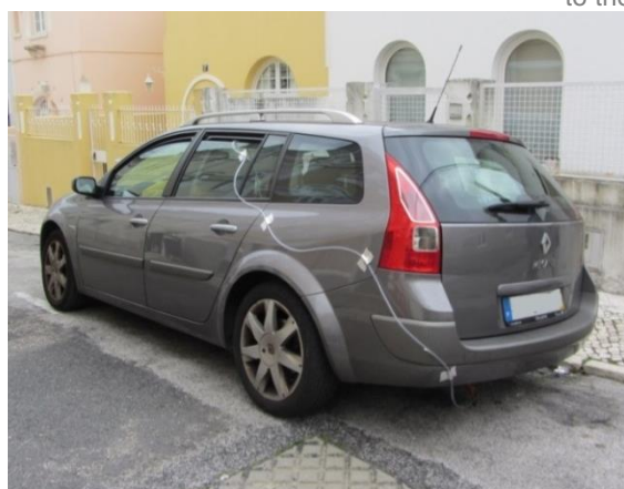
Figure 44 – Placement of the gas collecting tube between the tailpipe and the gas analyzer in the vehicle.
